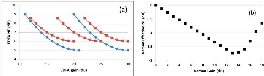
Figure 1: (a) EDFA NF in (dB) as a function of variable EDFA gain; dual-EDFA set (blue) and triple-EDFA set (red). (b): Raman noise figure as a function of Raman gain (after [11]).
