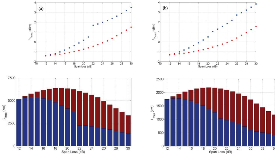
Figure 2(a,b):  $P_{Tx,opt}$  (dBm) versus  $L_s$  for EDFA-only (upper, blue) and hybrid Raman-EDFA (lower, red) dual (a) and triple (b) variable gain EDFA systems. Figure 2(c,d):  $L_{max}$  (km) versus  $L_s$  for PM-QPSK (c) and PM-16QAM (d) EDFA-only (lower, blue) and hybrid Raman-EDFA (upper, red) systems. Note VG EDFA-only stepwise transitions at 21dB (a,c) and 20/25dB (b,d)
